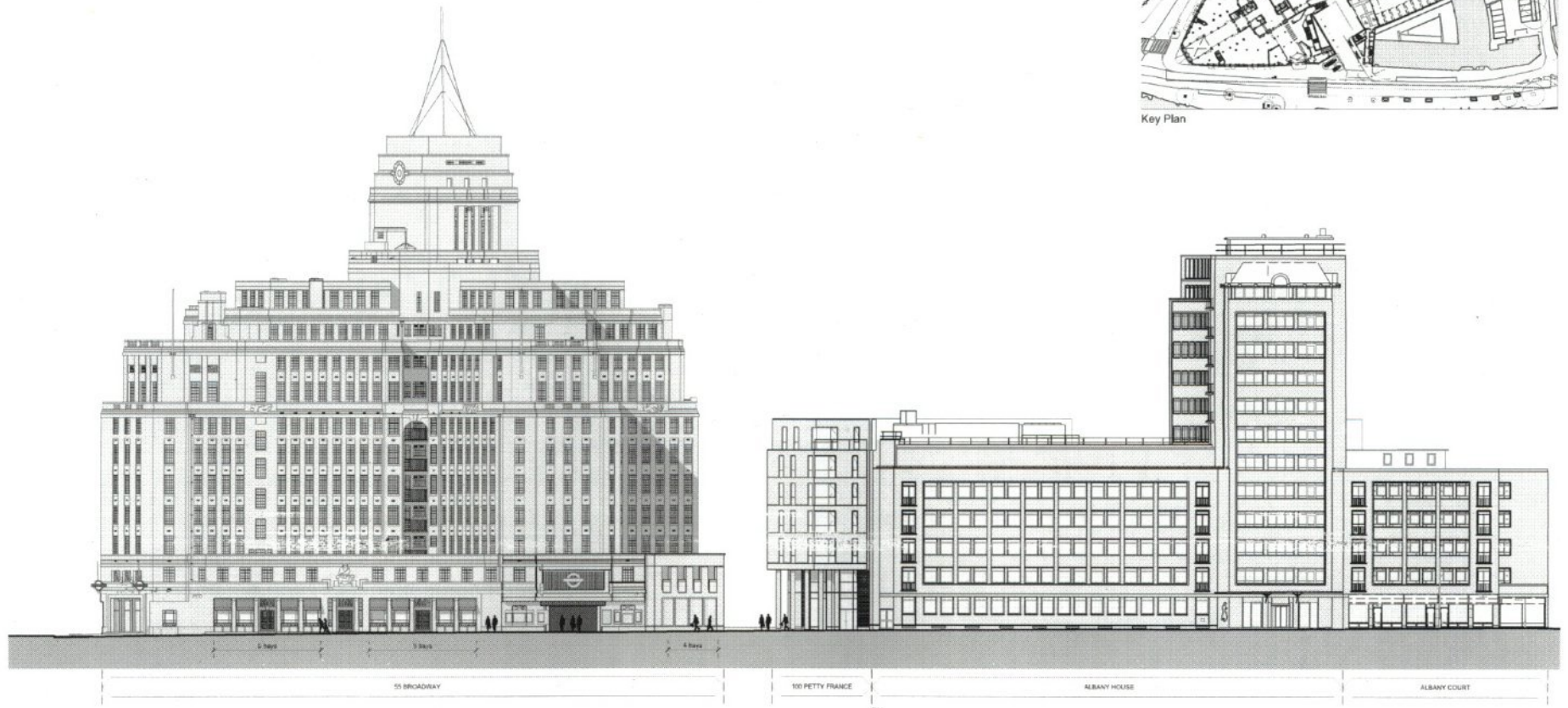
Proposed North Elevation - the italian intervention is to free the building of its immediate neighbour creating a logical separation of uses.
